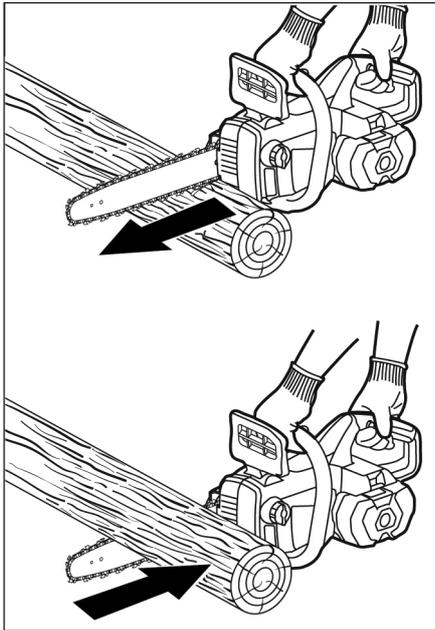
With drawing in, the chain saw is jerkily pulled to the workpiece.
