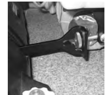
18 Slightly tighten the front push bars, do not tighten.
