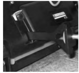
16 Reinsert the locking tabs and press them down until they lock.
