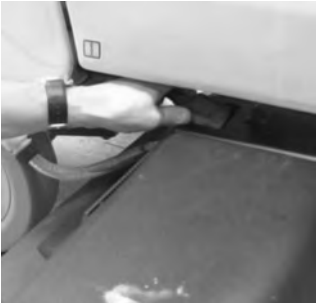
7 Install the connector tightly.
