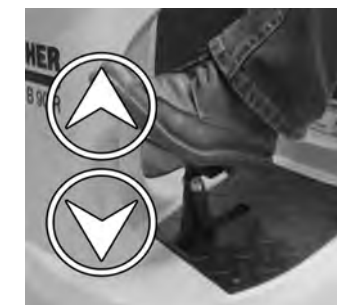
19 Check whether the brush head has been hooked in correctly. When you use the pedal to raise/lower the brush head, it must move freely.
