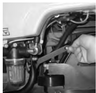
10 Press the side push bars toward the top.
