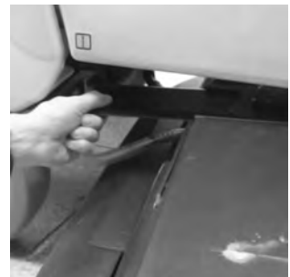
9 Close and lock the machine cover.
