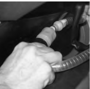
14 Create a water connection.
