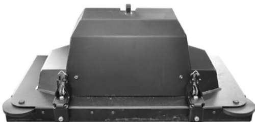
The installed holder at the front of the S65 oscillating head
