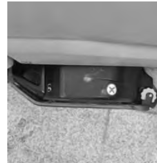
17 Align the brush head - exterior edge of the brush head must be parallel to the appliance frame.
