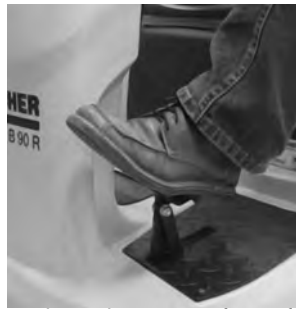
11 Press down the rear surface of the pedal to raise/lower the cleaning head, release and let the pedal move upwards.
