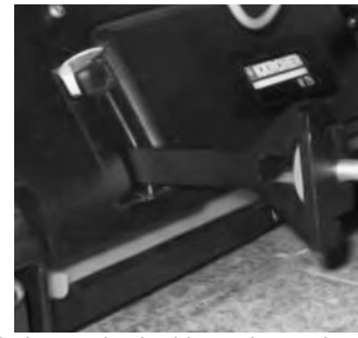
16 Reinsert the locking tabs and press them down until they lock.
