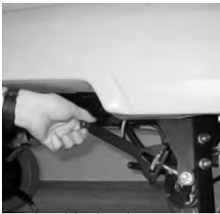
6 Move the side drawbars toward the top.
