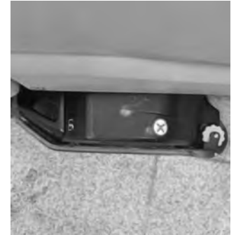
17 Align the brush head - exterior edge of the brush head must be parallel to the appliance frame.
