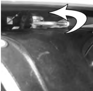
13 Rotate the holding pin to the left by 90° until it locks.
