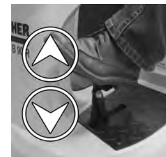
19 Check whether the brush head has been hooked in correctly. When you use the pedal to raise/lower the brush head, it must move freely.
