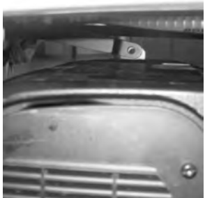
12 Position the centre holding bar in the bottom position and insert the holding pin.
