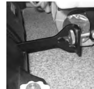
18 Slightly tighten the front push bars, do not tighten.
